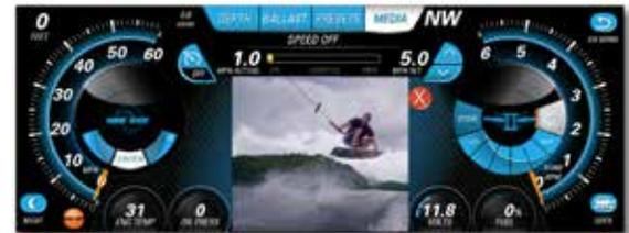
**Rear Camera:** With the back-up camera option turned ON in the Settings menu, the REAR CAMERA option will be available for selection.
