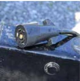
Malibu Trailers will integrate with most tow vehicle wiring harness requirements. Note the plug-in in the accompanying photo. If the harness will not connect to the plug, contact either the authorized Malibu dealer for assistance or the tow vehicle's authorized dealer. A different harness or an adapter may be necessary. These should be installed only by trained service technicians. Never use any harness or adapter that is not specified by the tow vehicle manufacturer and Malibu Trailers.
