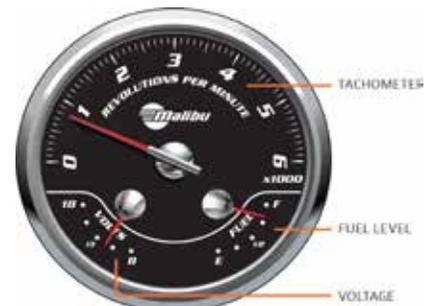
The lower right side of the gauge shows the approximate level of the fuel in the fuel tank. Note that movement of the boat can affect the reading, especially as fuel levels lower. Be certain to read the Fueling information in the Get Ready section of this Owner's Manual before operating the boat for important information
