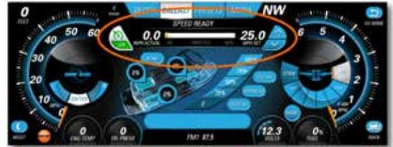
**Speed Input:** Press the SPEED INPUT button to access the screen below. Select the desired speed input source by pressing either PADDLE WHEEL or ZERO OFF-GPS. Changes will not take place until the throttle is put into the idle position.
