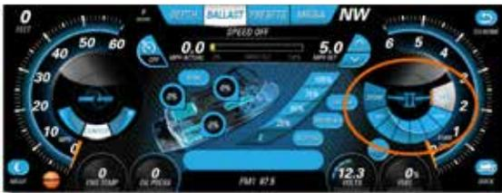
Before the ride begins, deploy the Power Wedge to a downward position by touching any one of the eight (8) position buttons on the Power Wedge control. If the wedge is in the stow position (all the way up), you can press any of the remaining piano keys to deploy the wedge.
