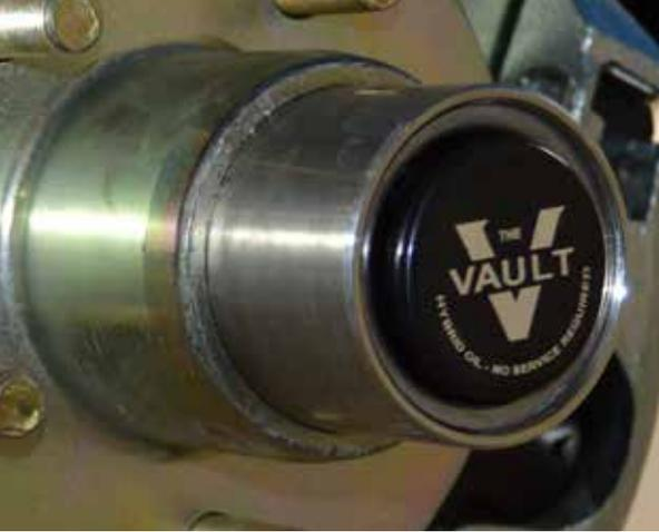
rear of the hub is sealed. The slight pressure inside the hub is needed to keep water out of the hub chamber when the hub is submerged underwater during loading and unloading.
