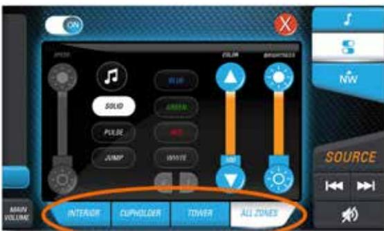
**Backlighting Zones:** The zone backlighting buttons, INTERIOR/CUPHOLDER/TOWER/ALL ZONES, allow each button to match the selected color and mode of that zone.
