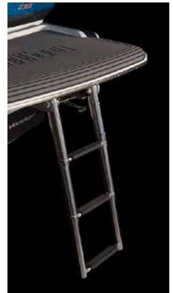
extended for use, and also for when it is folded up and put away. On the bow, the ladder folds upward and fits inside the anchor locker. The aft ladder folds up and under the swim platform for stowing. The ladders should always be stowed when the boat is underway. Excessive force of the body of water as the boat is in motion can damage the ladder, and such damage is not covered under warranty.
