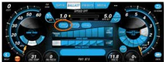
**Wake View:** The Wake View screen provides a simplified wake control interface. Use the BOAT/WAKE VIEW button to switch between modes.
