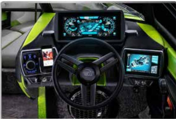
The Malibu dash features two video screens, through which most of the functionality of the boat operation is controlled. On the lower left will be either the standard storage area or the optional Sport Dash, which is explained in the How It Works section of this Owner's Manual, as well as in this section.
