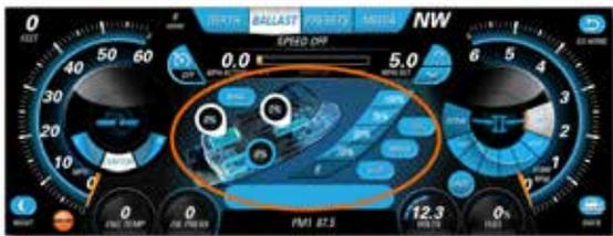
**Boat View:** Choose the perfect ballast combination to create a custom wake. The Ballast screen displays tank levels and provides controls to fill and drain the tanks.
