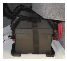
Because batteries contain fluid that is caustic and potentially dangerous to skin and body parts, boat operators need to ensure that the batteries are securely in place. Also, if the connections are loose, erroneous readings may be sent to the boat system, which can
