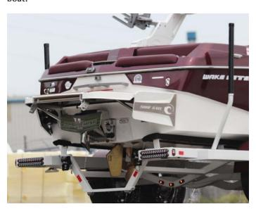
Then you should release the tie-downs except the winch. Slowly back the trailer and boat into the water. If possible, have a second person standing by (but never directly in back of the rig) to help guide you. When backing up, note that the trailer will go in the opposite direction to the direction in which the tow vehicle steering wheel is turned.
