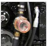
To protect the system, a sea strainer is installed near the raw water intake and serves the purpose of keeping debris from entering the cooling system, causing eventual engine failure. As with any kind of strainer, it is necessary to regularly clean it so that water can flow unimpeded.
