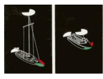
Figure 1 Motorboats less than 20 meters (65.62 feet) shall exhibit avigation lights as shown. (Note: Two masthead lights are
