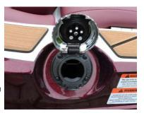
Malibu strongly recommends use 93 octane top tier detergent gasoline. The additives and detergents in these fuels can reduce the amount of buildup in the engine that adversely affects performance and shortens the life of an engine. Retailers selling top tier gasoline can be found at www.toptier.com. (This information points to a palletizing company so needs to be removed or replaced with new recommendations.)
