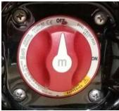
**Four-Position Isolator System.** Because of the electrical requirements to enjoy the Malibu boat in its fullest experience, most models are equipped with two (2) batteries. The optional battery ON-OFF switch is located in a panel behind a door on the port side of the walkthrough between the bow and center deck.
