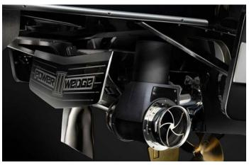
speed is above 1 mph and below 10 mph. Always verify there is no person or object around the Power Wedge while it is stowing. If an object is obstructing the process, damage or injury could occur if caught between the wedge and the transom. The Power Wedge III has a pressure relief valve to allow the wedge to move manually and freely in the event of a fault. Information on how to use the pressure relief valve is provided in the *Care and Maintenance* section of this manual.
