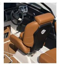
Boat owners can also order a power option that allows the driver's seat to be moved up or down by pressing on a slide button on the starboard side of the seat base at the shifter panel. Pushing up moves the seat up; pushing down moves the seat down. All driver's seats have a mechanical lever to allow the seat to slide forward and aft, explained above in the *Seating* section.
