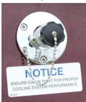
onshore. Run a garden-type hose from the clean water source to the inlet on the port side of the deck, outside the engine storage compartment. Attach securely, but do not overtighten.
