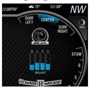
Touch Backlighting to allow the driver to adjust the brightness of the 12", 7", and dash LEDs from 1% to 100%. There are two modes for the system backlighting: automatic and manual.
