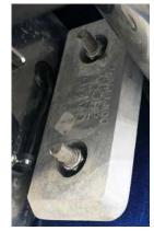
of the body of water than that occurring between the boat's metal parts and the water. Simply, both rust (which is oxidation) and metal reduction are the result of operating in salt water, and the anodes' purpose is to attract and draw away much of the corrosion from the boat's metal components.
