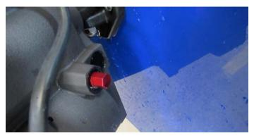
For the Power Wedge III, using a small (stubby) straight screwdriver, loosen a small red screw on top until it stops. Lift or lower the wedge to the position desired and then tighten the screw snugly (but do not over-tighten). Manually cycle the wedge a couple of times after doing this to ensure that the screw is snug, and the wedge moves correctly.
