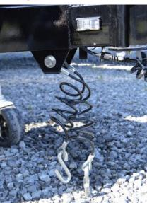
The safety cables can prevent a trailer from totally disengaging from the hitch. If it becomes necessary in the future to replace the cables, ensure that the replacement cables meet the Society of Automotive Engineers (SAE) J684 standard for trailer hitching and coupling. The cables must match or exceed the trailer's GVWR.
