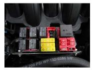
In addition to the circuit breakers that control the majority of electrical activity on the boat, Malibu engines also have a fuse box on the engine. See photo left.
