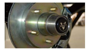
Vault uses only Hybrid Oil™ lubricant, which combines the benefits of oil and grease. The Vault protects the wheel bearings in a sealed, pressurized chamber that is unaffected by outside elements. For optimal performance, only UFP's Hybrid Oil Lubricant should be used in this system.
