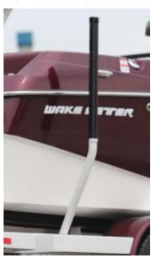
Malibu trailers are equipped with removable guide poles as standard equipment. The poles, located on each side of the trailer, assist in assessing the total width of the boat and trailer relative to towing or while backing up, as well as parking the trailer and boat inside shelter such as a garage.
