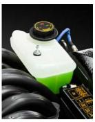
grade coolant (such as Sierra) and clean, distilled water. (Some brands sell coolant conveniently premixed. Be sure to read the label carefully, and do not add any water to coolants that are premixed. This will dilute them to unacceptable levels of mixture.) When mixing coolant and distilled
