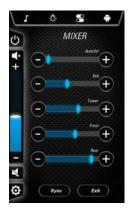
The Equalizer page allows the driver to adjust the treble, mid, bass, and balance. It is recommended to leave the treble, mid, and bass centered at zero.
