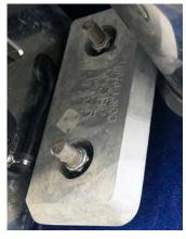
are the effects of operating in saltwater. To reduce these naturally occurring results on boat components, the sacrificial anodes attract and reduce most of the effects.
