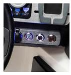
On a boat equipped with a Start-Stop button, press the button. If you are using the backup key, also turn the key to OFF. (Failing to do so means the electrical system will continue to function; eventually, this will drain the battery or batteries.)
