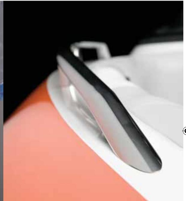
**twelve. Oval Bow Rails and Safety Handles** All Malibu bow rails and safety grab handles have been designed with an oval shape for added safety and pleasing aesthetics.
