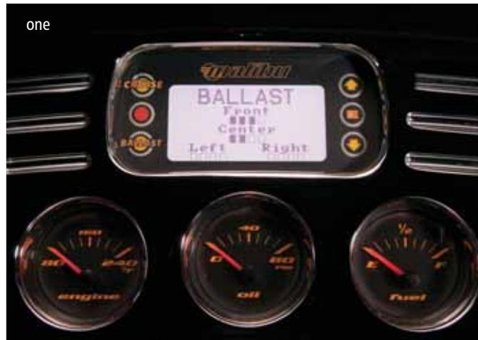
**one.** The Ballast Monitoring System data, which enables you to track and duplicate individual wake preferences, is now easily visible in the centered LCD graphical dash display, featuring a bar graph that shows ballast volumes in each tank.
