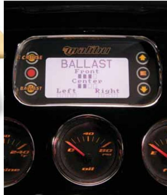
**fifteen. Ballast Monitoring System (WVLX, W23LSV, W23XTi, W247LSV only)** Malibu's industry-exclusive graphical information center monitors and displays the volume of each ballast tank, providing each rider with the ability to customize wakes for their own riding style.
