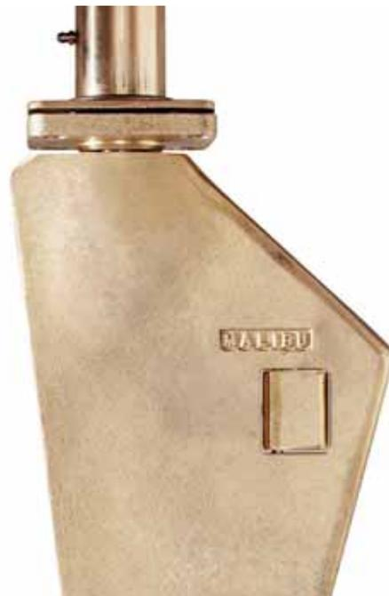
**six. Adjustable Rudder** Another first introduced by Malibu is the ability to fine tune the rudder for a personal preference on rudder torque. The adjustable rudder is standard on every Malibu boat.
