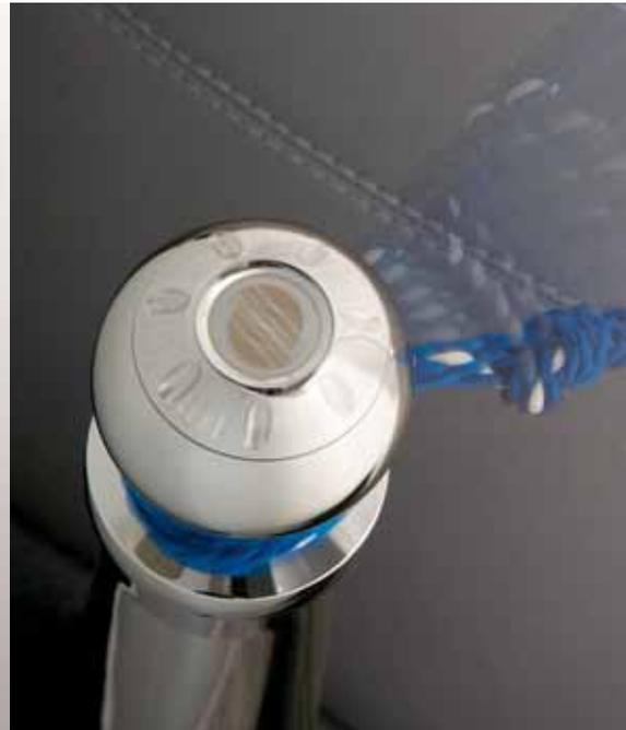
**eleven. Patented Swivel-Head Pylon** Malibu's patented swivel-head pylon rotates on precision bearings. The seamless rotation eliminates ratcheting and rope wear for a smoother, safer tow and longer rope life.
