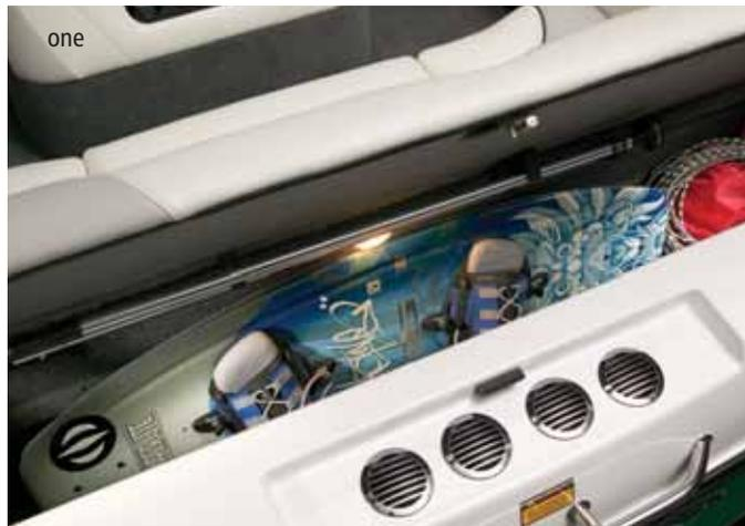
**one.** The iRide has an additional storage trunk near the transom, with a helpful light feature, for tucking away boards and skis.
