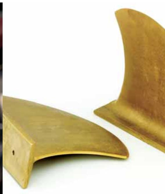
**three. Gorilla Tracking Fins** Malibu's Gorilla fins enhance the handling stability and tracking capabilities of Sport-V configured boats. Larger surface areas and a more stable center pivot point increase the boat's overall dynamics and provide direct drive maneuverability.
