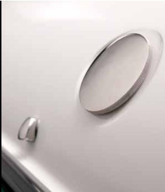
**ten. Dual Gas Fills** Dual gas fills emptying into one central tank are standard on every Malibu boat for a more convenient refueling experience.
